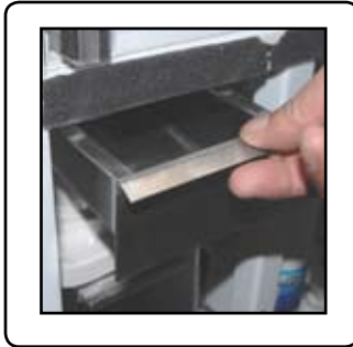
Fig 18 Replacing Drip Tray
