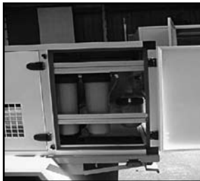
Water Filtration Unit
