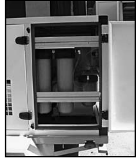
Water Filtration System
